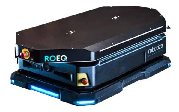
The ROEQ TMC300 top module is designed for the Robotize GoPal P35 to transport the ROEQ Cart500. With this cart solution the Robotize GoPal P35 can safely pick up, transport and drop off cargo of up to 300kg.
